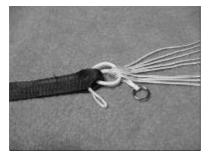
3. Wrap-It<sup>TM</sup> through lines and riser a **second** time...
