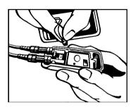
Disconnect the power pack by holding the connector by its small edges. Be careful not to pull on the wires.
