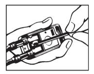
Partially unscrew the printed circuit fixing screw with three complete turns only. Do not remove the screw from the printed circuit board. Do not remove the printed circuit board from the case.
