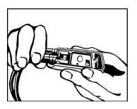
By pushing the two connectors upwards it is possible to lift the printed circuit slightly.
