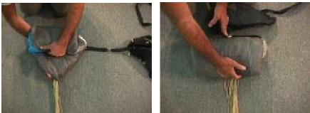
Keep the roll tight and maintain the width of the bag. The bridle needs to be pulled far enough from the center of the roll that it can be wrapped around the outside of the roll and maintain contact with the grommet in the deployment bag.
