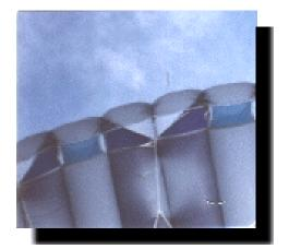
The Icarus EXTreme's cross-braced tri-cells are the key to its ultra-high performance.
