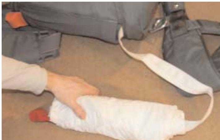
Grip firmly the folding drogue chute and stow it into the spandex pouch.
