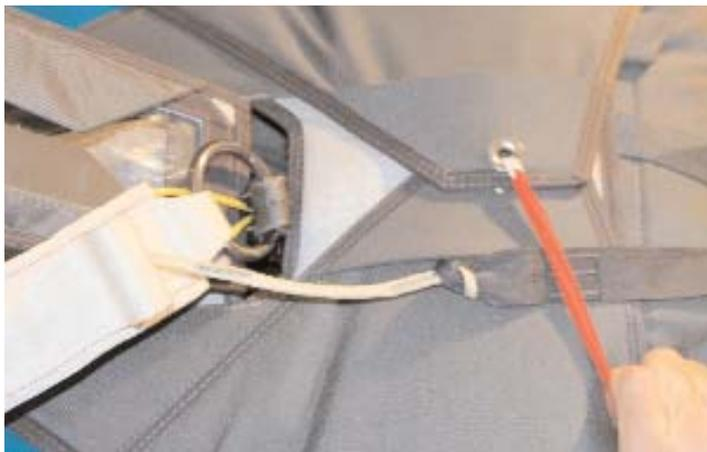
Droque chute setup must be as shown on both below photos. The inner kill line bridle is oriented toward the main container.
