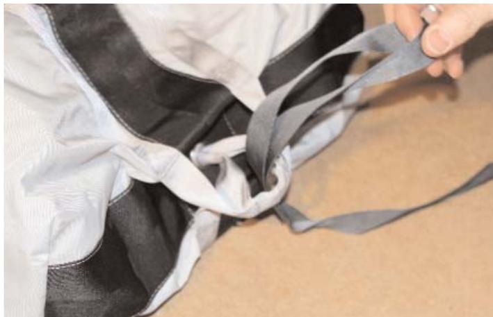
4° Route the complete Drogue Chute through the lower end loop and squeeze the knot.
