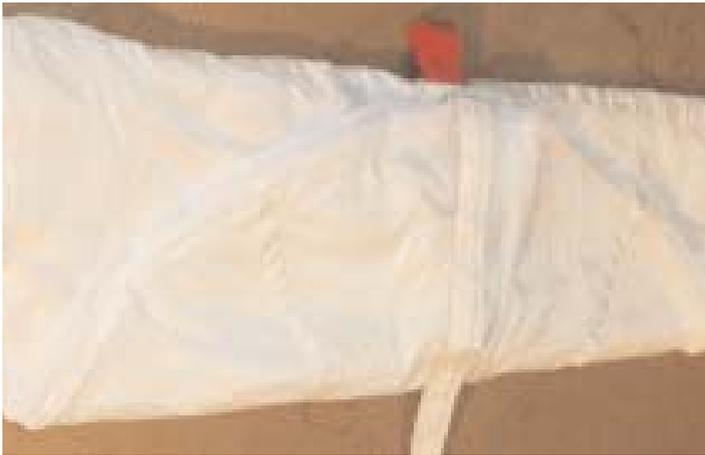
Fold the pilot chute toward the handle and fold the bridle over.
