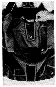
4. Thread the Release Unit through the bottom passage hole of the spandex pocket and then through the tape channel to the No.1 reserve side flap. Trimming of the tape channel may need to be done at the side flap end to ensure no snagging during deployment.
